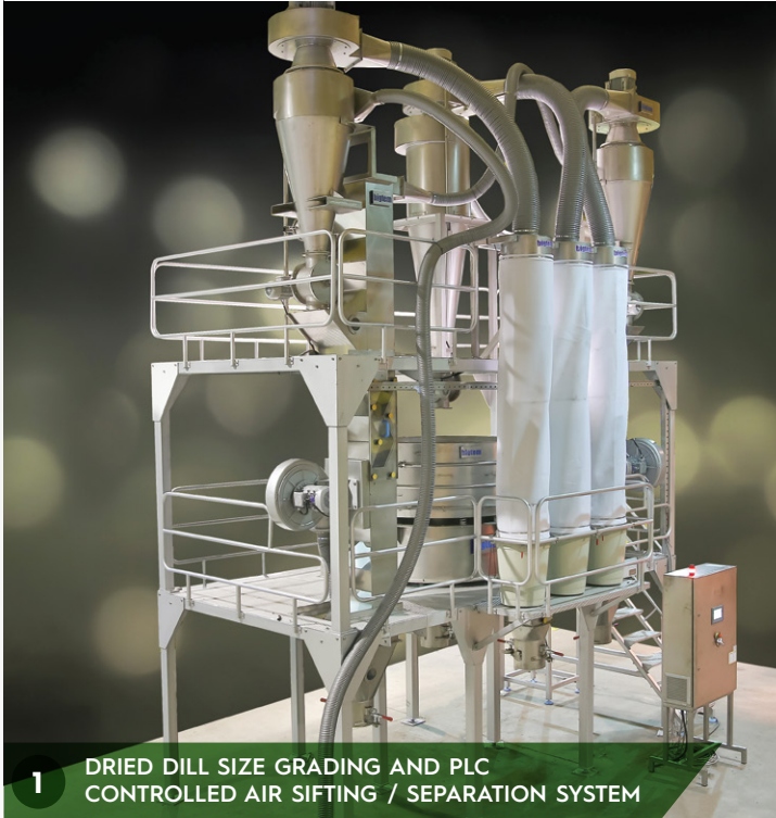
2 AIRFLOW CONTROLLED DILL SEPARATION SYSTEM
